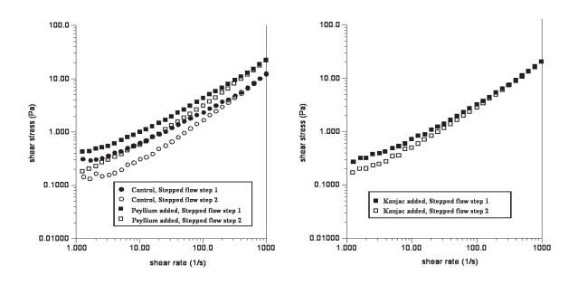
Figure 2. Flow behaviour of acid-thinned starch suspension with or without konjac or psyllium added.
