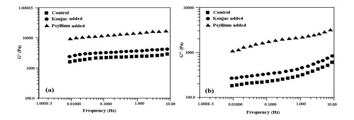
Figure 1. Variation of storage modulus (G') and loss modulus (G") as a function of frequency
